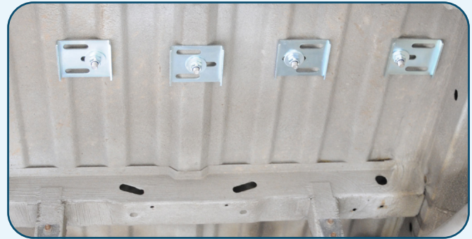
View from underneath vehicle with lock plates
