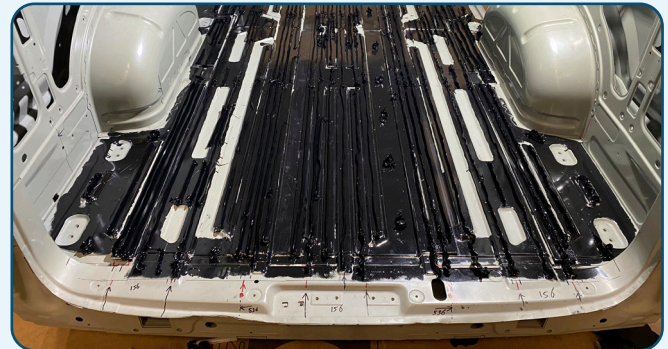
Sikaflex 268 / Sika 268 PowerCure applied to the vehicle floor.
