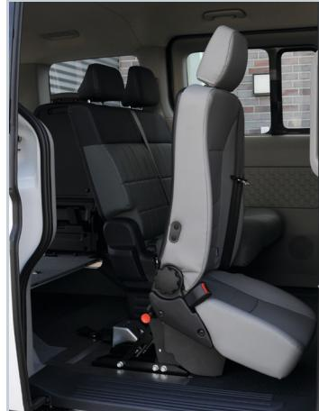
For easy access to the passenger compartment, the seat at the side entrance can be folded forward.
