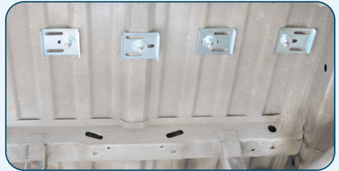
View from underneath vehicle with Lock Plates
