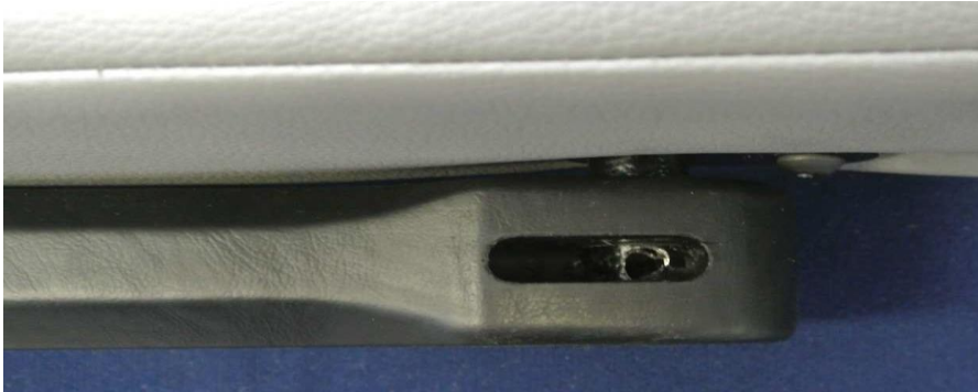
Picture 7. Armrest assembled to the seat.
