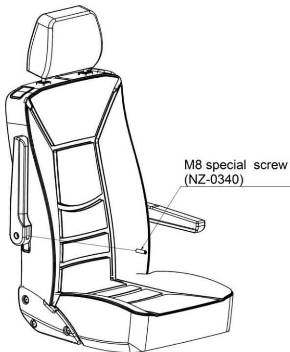
Picture 8. M8 special screw in armrest adapter.
