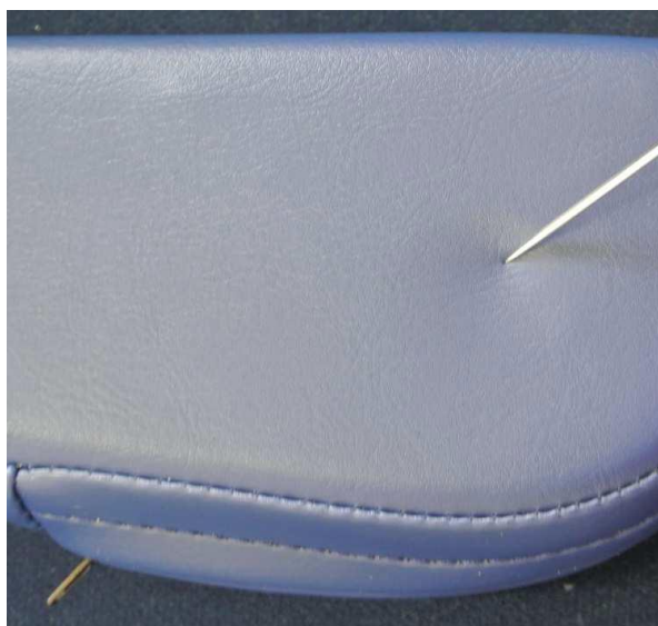
Picture 10. Signify holes in a upholstered armrest.
