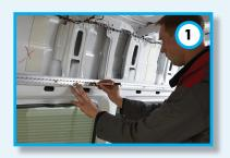
1. Carefully **remove** the interior trim and head lining. Mark the drill holes for the mounting plates with the matching bolts. Use the rail to mark the spots. Please **ensure** that the rail is in the correct position. The location of the holes differ **front** to rear.
