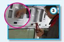
3. Slide the mounting plate in place. Line up the hole of the mounting plate with the hole which has just been drilled of 11 mm. Mount the rivets and unscrew the bolt.
