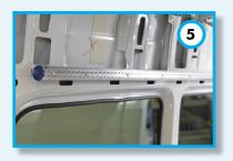
5. Mount the rail with the stainless steel bolts (**provided**) M8 x 50 mm A2 class 70. **Fasten the bolts with maximum torque 20 Nm**. (Side Trim and head lining not visible in the picture.)
