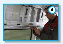
4. Make holes in the head lining for the spacers. Fit the side trim and head lining. Use the provided spacers to clear the space between the bodywork and the side trim and headlining. (Side Trim and head lining not visible in the picture.)
