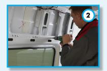
2. Drill a hole of 11 mm in the upper part of the bodywork above the window. Use the mounting plate to define the holes for the rivets. Drill the defined holes with a 4.2 mm drill.
