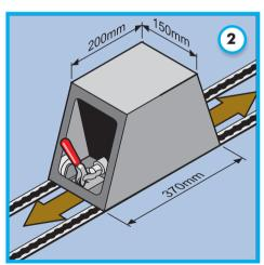
Slide along the floor tracking to any position and stop in your required location.
