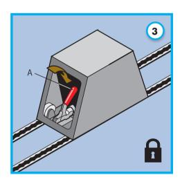
Clamp Safebase in position by pushing clamp handle forwards into the Safebase. The Safebase is now locked.
