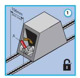
To unlock the Safebase to slide on the floor tracking, pull clamp handle A away from the Safebase.
