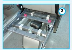
3. Mount the chair to the Smartlegs Legs using the mounting brackets and hex bolts. Quality 10.9 or higher nuts and bolts. First mount all nuts and bolts before securing them. Secure these bolts with a minimum torque of 20 Nm.
