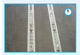
1. Place the M8 T-Bolts in the rail, then place the single T-Bolt at the front and the double T-Bolt 95mm at the rear.
