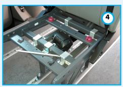
4. Mount the chair to the fixed legs using the mounting brackets and hex M8x45 nuts and bolts of quality 10.9 or higher. First mount all nuts and bolts before securing them. Secure these bolts with a minimum torque of 20 Nm.
