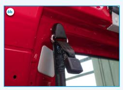
Mounting of the seatbelt retractor (C) behaving the wheel arch
