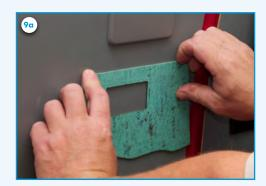
9a) Mark a rectangle of 35 x 64 mm for letting the seatbelt go into the vehicle from behind the side trim.
