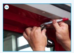
14a) Determine the correct position of the upper seatbelt anchorage point which is as straight as possible above the upper seatbelt anchorage point above the window.
