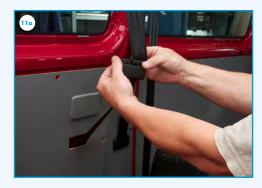
11a) Make a small cut in the side trim seatbelt cover (G). Pull the seatbelt into the side trim cover and mount the cover on to the side trim.
