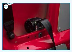
13a) Mount the seatbelt retractor with bolt (B).
