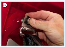
5a) Mount the upper seatbelt point with the corresponding bolt 7/16" UNF 8.8 which is in the mounting kit.
