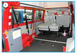
1) The positions of the seatbelt retractor and the upper belt point are free of choice along the indicated line for mounting. Make sure that the retractor and the upper belt point are as vertical as possible.
