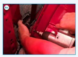
8a) Mount the retractor of the seatbelt with bolt (B) to the bodywork as shown.
