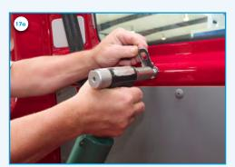
17a) Mount the seatbelt tongue with the rivets (I).
