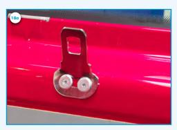
18a) Bend the seatbelt tongue a little bit if necessary.
