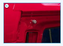
4a) Mount the mounting plate with the rivets (F). Remover the bolt and mount the side trim.
