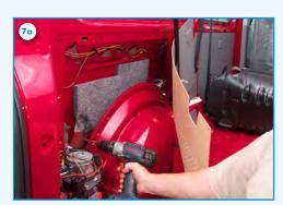
7a) Drill a hole of 10.5 mm in the bodywork of the vehicle for mounting he retractor as shown in the picture.
