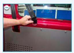
16a) To prevent swinging of seat belts which are not in use a seat belt tongue can be mounted.
