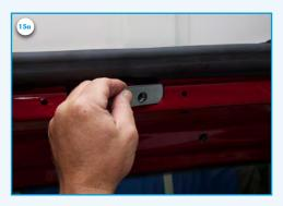
15a) Use the mounting plate (E) for marking the holes for the rivets. Drill the holes for the rivets with a 4.2 mm drill.
