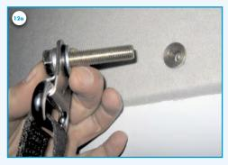
12a) Mount the upper seatbelt point with the bolt (E).
