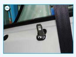
13a) To prevent swinging of seat belts which are not in use a seatbelt tongue can be mounted. Drill two holes of 5.1 mm for mounting the seatbelt tongue (H). Mount the seatbelt tongue with the rivets (I). Bend the seatbelt tongue a little bit if necessary.
