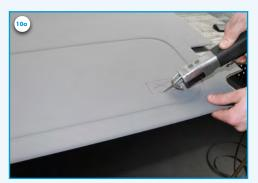
10a) Cut a rectangle hole of 35 x 64 mm in the side trim. Unscrew the upper seatbelt point and guide the seatbelt through the rectangular hole.
