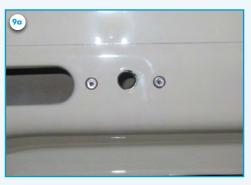
9a) Mount the rivets (F). Unscrew the bolt and mount the side trim and head lining. Use the provided spacers to clear the space between the bodywork and the side trim and headlining.
