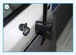
11a) Make a cut in the side trim seatbelt cover and slide it over the seatbelt.
