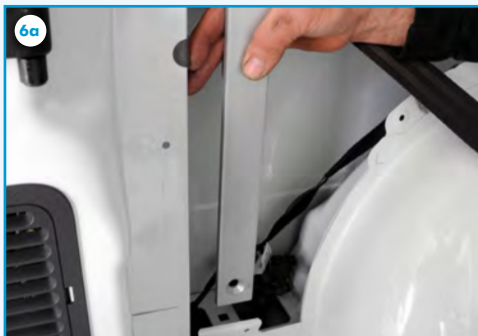
6a) Stick the metal strip (A) through the long hole.
