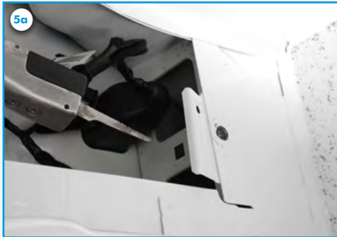
5a) Saw the metal between the two holes so you will end up with a long hole.
