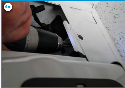
4a) Drill two holes behind the vertical edge.
