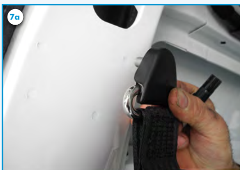
7a) Drill a hole of 11 mm as straight as possible in a vertical line above the retractor. Drill the hole in the upper part of the body. Above a window or in the D column as shown in the picture.
