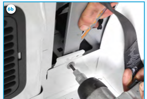
6b) Screw the metal strip (A) with the counter sunk screw (B) M10x20 into the vehicle.
