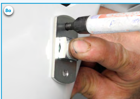
8a) Use the upper seatbelt point mounting plate (E) for defining the holes for the rivets.
