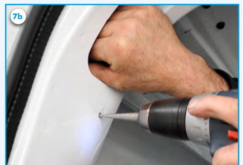
7a) Drill a hole of 11 mm as straight as possible in a vertical line above the retractor. Drill the hole in the upper part of the body. Above a window or in the D column as shown in the picture.
