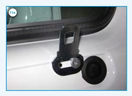
11a) To prevent swinging around of the seat belts a seatbelt tongue can be mounted in the body under the window. Drill two holes of 5.1 mm (H). Mount the seatbelt tongue with the rivets (I). If necessary the seatbelt tongue can be bent.
