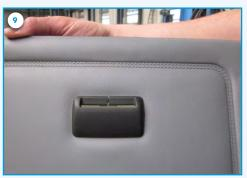
9) Make a cut in the seatbelt side trim cover (G) and let the seatbelt go through the cover. Mount the cover in the rectangular hole.
