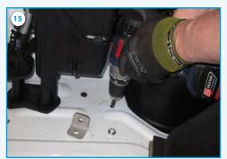
15) Drill a hole of 10.5 mm in the floor of the vehicle.
