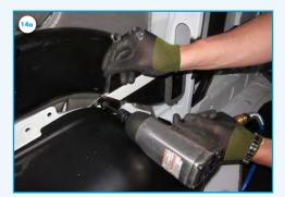
14a) Mount the metal bar with the bolts (B)  $M8 \times 20$  mm.
