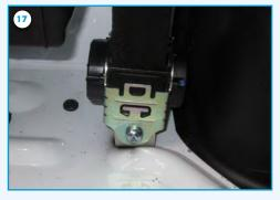
17) Mount the seatbelt retractor (C) with the hexagon bolt M10 x 25 to the bracket.
