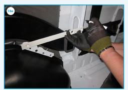
13a) Define the holes to drill with the metal bar (A). The metal bar should be mounted above the outflow opening of the air-conditioning.
