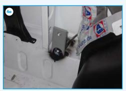
4) Mount the seatbelt retractor (C) with the hexagon bolt (D) to the metal bar (A).
