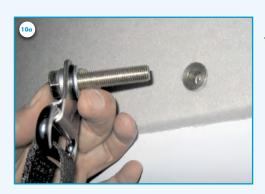
10) Mount the upper seatbelt point (K) to the upper seatbelt anchorage point.
